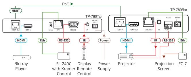
Figure 6: Connecting TP-789R/TP-789Rxr as PoE Acceptor
