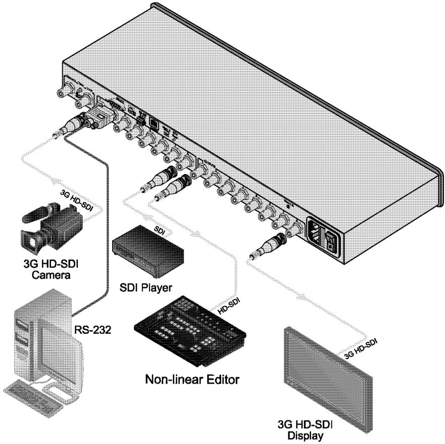
Figure 2: Connecting the VS-88HDxl 8x8 3G SD/HD-SDI Matrix Switcher
