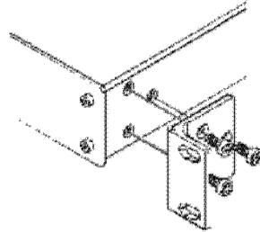
2. Place the ears of the machine against the rack rails, and insert the proper screws (not provided) through each of the four holes in the rack ears.
