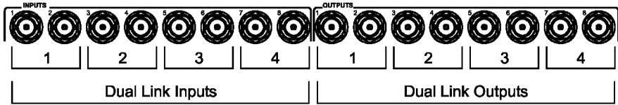
Figure 3: VS-88HDxl Dual-Link Inputs and Outputs
