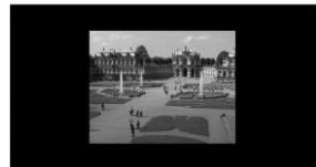
**FOLLOW OUTPUT** – The aspect ratio and resolution of the input signal is re-sized to precisely match the aspect ratio and resolution of the **VP-773** output signal. This may result in some distortion to the input signal images
