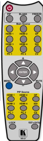
Press the PIP button (to access the PIP mode) and then press one of the 8 INPUT (PIP Source) buttons to select the PIP window
