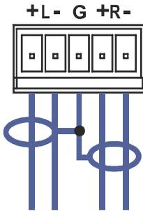
Figure 6: Connecting the Balanced Stereo Audio Output
