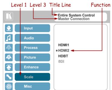
If the display layout includes a PiP window, you can set the OSD menu to control the main source window and the PiP window separately (by defining Window Control, see [Section 6.8](#)).
