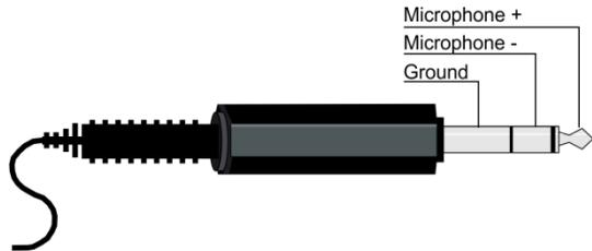
Figure 8: Microphone Pinout
