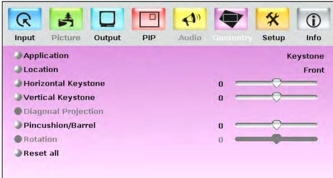
Figure 20: Geometry Screen
