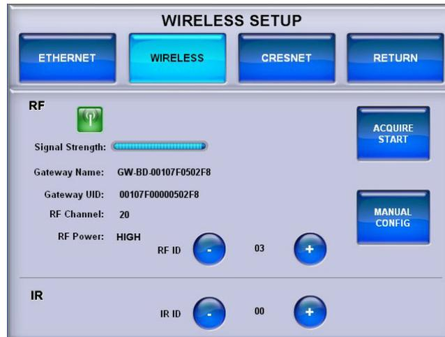
The WIRELESS SETUP menu displays RF connection status, signal strength, gateway name and UID, RF channel and RF power settings. – and + controls are provided to set the *RF ID* and *IR ID*.
