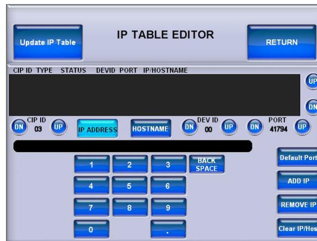
The *IP TABLE EDITOR* offers the option of entering the information as an IP address (as shown in the illustration above) or as a hostname (as shown in the following illustration). Simply touch **IP ADDRESS** or **HOSTNAME** to switch between the two methods.
