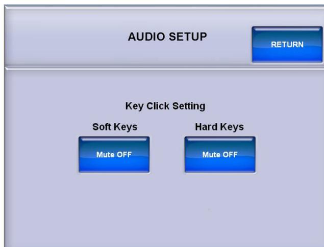
The AUDIO SETUP menu offers a pair of buttons that allow muting of the key click sound for either the *Soft Keys* (on screen buttons) or the *Hard Keys* (buttons on the front of the touchpanel).
