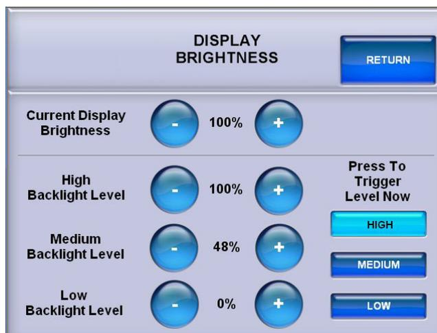
The DISPLAY BRIGHTNESS menu provides – and + controls to adjust *Current Display Brightness*, *High Backlight Level*, *Medium Backlight Level* and *Low Backlight Level*. These last three are the brightness levels the display will be set to as the right trigger key (on top of the touchpanel) is used to toggle between high, medium, and low screen brightness, provided *Trigger Key Control for Screen Brightness* is set to **ON** in the BACKLIGHT SETUP menu.
