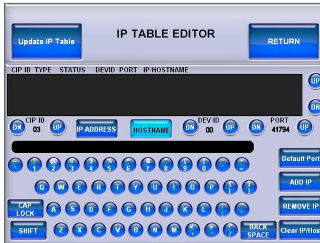
To add an IP address (or hostname), use the **DN** and **UP** buttons to select the *CIP ID*. Then use the numeric keypad on the screen for IP address entry or touch **HOSTNAME** to switch to the alphanumeric keypad. When both the *CIP ID* and IP address (or hostname) have been entered, touch **ADD IP** to add the entry to the list.
