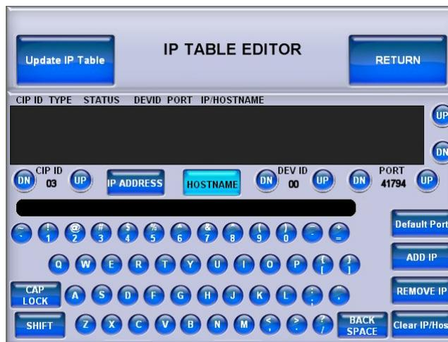
To add an IP address (or hostname), use the **DN** and **UP** buttons to select the *CIP ID*. Then use the numeric keypad on the screen for IP address entry or touch **HOSTNAME** to switch to the alphanumeric keypad. When both the *CIP ID* and IP address (or hostname) have been entered, touch **ADD IP** to add the entry to the list.
