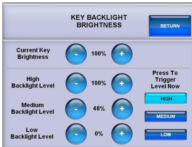
The KEY BACKLIGHT BRIGHTNESS menu provides – and + controls to adjust *Current Key Brightness*, *High Backlight Level*, *Medium Backlight Level* and *Low Backlight Level*.
