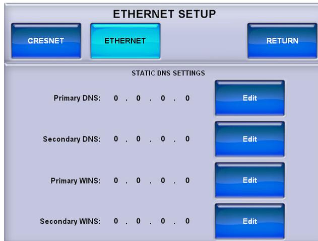
From the **STATIC DNS SETTINGS** menu, touch the **Edit** buttons to enter the menus that allow you to set the *Primary DNS*, *Secondary DNS*, *Primary WINS* and *Secondary WINS*, as shown in the following illustrations. + and – buttons on each menu are provided for setting the numbers. In each case, touch **RETURN** to go back to the previous menu.
