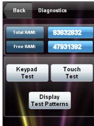
The “Diagnostics” screen displays information about the *Total RAM* and *Free RAM* in your TPMC-3SM or TPMC3SMD. It also provides **Keypad Test**, **Touch Test** and **Display Test Patterns** buttons to access the “Keypad Test”, touch test and “Test Patterns” screens, respectively.
