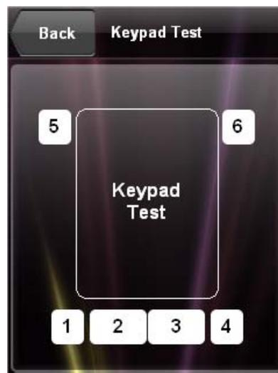
The “Keypad Test” screen can be used to test the function of the four hard key push buttons below the screen and the two backlit buttons on either side of the top of the
