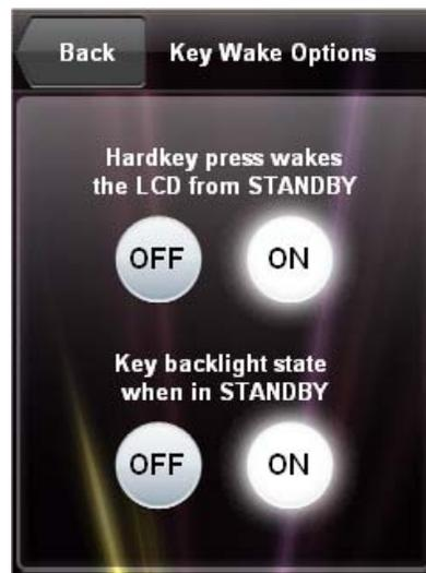
This screen provides controls for turning the *Hardkey press wakes the LCD from STANDBY* and *Key backlight state when in STANDBY* functions **ON** or **OFF**. Touch **Back** to return to the “Standby Timeout” screen, then touch **Back** to return to the “Panel Setup Options” screen.
