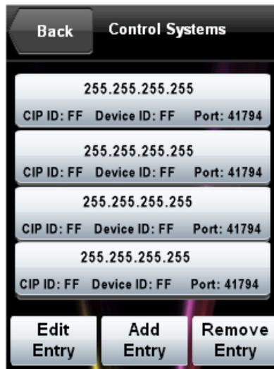
The “Control Systems” screen provides information about IP addresses, *CIP ID*, *Device ID* and *Port* for up to four entries.
