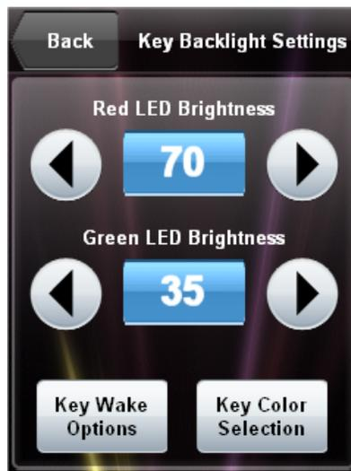
The “Key Backlight Settings” screen provides controls for *Red LED Brightness* and *Green LED Brightness*. There is also a **Key Wake Options** button for accessing the “Key Wake Options” screen, shown at the bottom of page 7 and a **Key Color Selection** button for accessing the TPMC-3SM’s “LED Color Settings” screen, shown in the illustration at the top of the following page.
