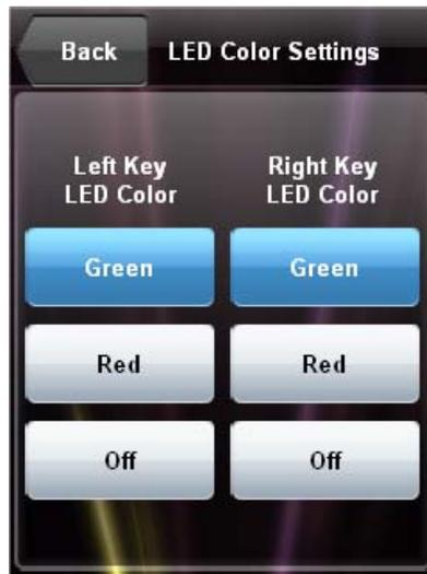
The TPMC-3SM’s “LED Color Settings” screen provides control for selection of *Left Key LED Color* and *Right Key LED Color* as well as controls for turning each of the LEDs **Off**.
