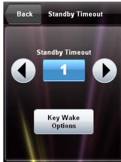
The “Standby Timeout” screen provides controls to adjust *Standby Timeout* from 0 to 120 minutes. Touch **Back** to return to the “Panel Setup Options” screen or touch **Key Wake Options** to display the “Key Wake Options” screen, shown in the following illustration.
