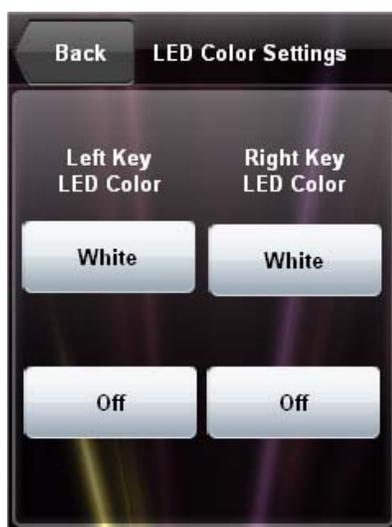
The TPMC-3SMD’s “LED Color Settings” screen provides control for selection of *Left Key LED Color* and *Right Key LED Color* (i.e., the **White** button turns the LED on) as well as controls for turning each of the LEDs **Off**.
