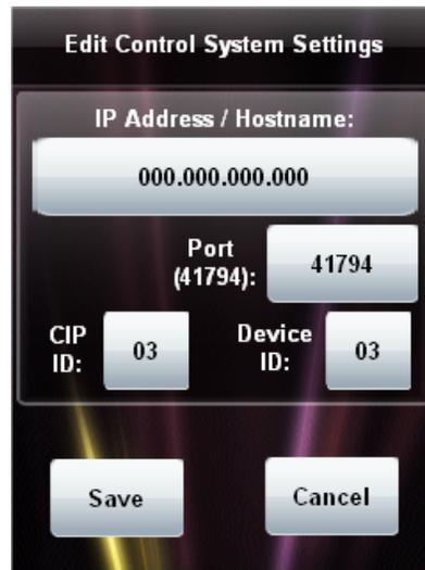
Touch the *IP Address / Hostname*, *Port*, *CIP ID* and *Device ID* fields to make each entry. Each will open an on-screen keyboard appropriate for the field. For example, touching the *IP Address / Hostname* field will open the keyboard shown in the following illustration.
