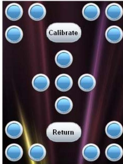
The touch test screen contains a **Calibrate** button to initiate touch screen calibration and a **Return** button to return to the “Diagnostics” screen.
