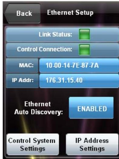
The “Ethernet Setup” screen displays information about your *Link Status*, *Control Connection*, Mac and IP addresses. There is a button to enable/disable *Ethernet Auto Discovery* and buttons that provide access to **Control System Settings** and **IP Address Settings**.
