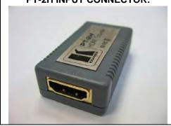
The **PT-2H** output is connected via a second male-to-male HDMI cable (not provided) to an HDMI acceptor, such as a projector or plasma.
