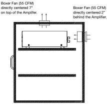
If the cabinet rear is not open to fresh air or if you're using low impedance loads, install two "boxer fans" to provide continuous air flow into and out of the cabinet.
