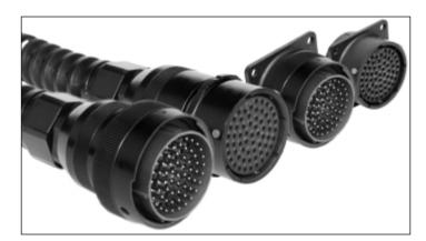
Amphenol's Multipin MP-62 series of circular connectors utilise the same design principles of the Mil-C-26482 military connectors. Featuring a three point quick mating bayonet coupling and five key polarisation ensuring a positive connection every time. Available in two contact pin layouts 39 and 61 with gold plated solder contacts fitted as standard.
