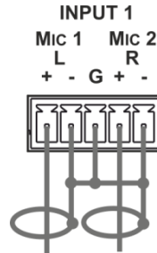
Figure 5: Connecting an Unbalanced Stereo Audio Source to the Input
