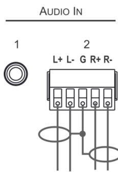
To an unbalanced stereo audio source:
