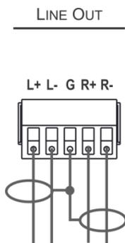
To an unbalanced stereo audio acceptor:
