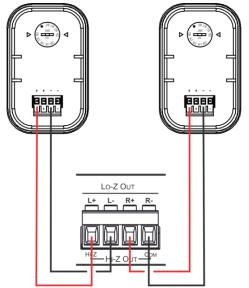
The following diagram displays the **Galil 6-AW** speakers connected to a recommended Kramer power amplifier (for example, **PA-120Z**):
