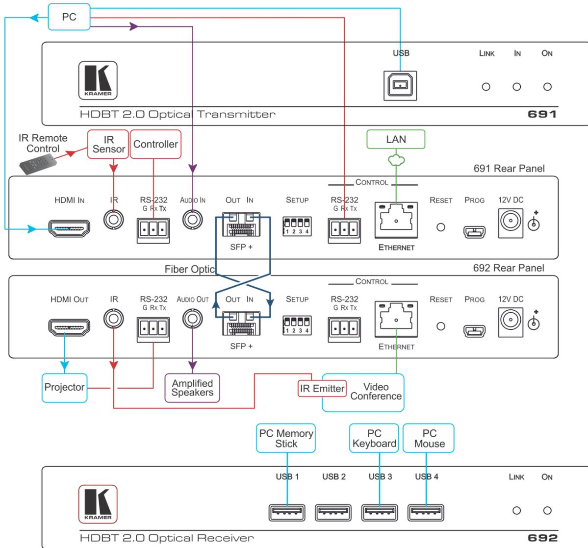
Always cross-connect the fiber connections, Rx OUT to Tx IN and Rx IN to Tx OUT, as transmission is carried on simplex fiber strands.
