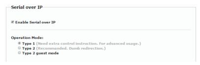
Figure 30: Serial over IP - Type 1 Operation Mode
