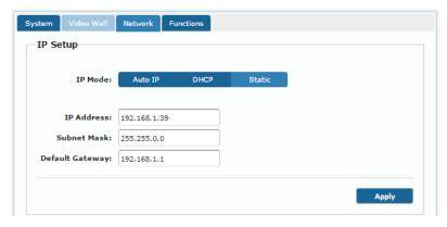
Figure 22: Network Tab - IP Setup
