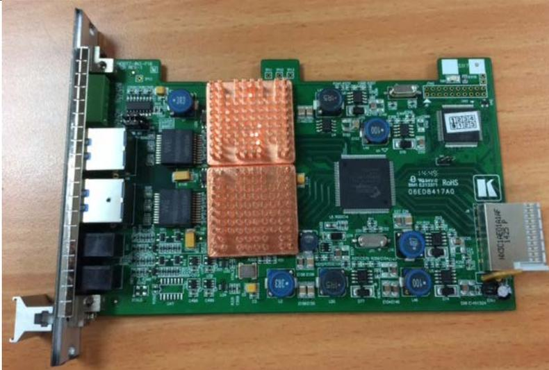
With enlarged heat dissipation radiators, **any number** of HDBT and HDBT7 IN and OUT cards can be installed in a VS-1616DT frame.
