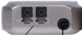
2 Strand LC-LC Fiber Optic Cable Input
