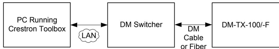
DM-TX-100/-F connects to DigitalMedia switcher via DM network:
