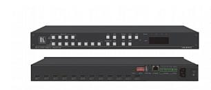
VS84H2 is a highperformance 8x4 matrix switcher for 4K@60Hz (4:4:4) HDR signals and digital audio routing. It reclocks and equalizes the signals and can route any one of 8 HDMI, HDCPcompliant sources (selectable) to any or all outputs simultaneously. VS84H2 offers unmatched audio flexibility where any embedded digital audio input can be routed to any digital output in addition to four ARC sources to produce an equivalent 12x8 audio matrix
