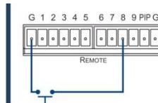
Figure 30: Connecting the Contact Closure Remote Control PINs
