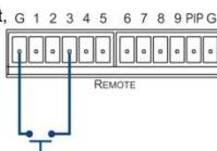
To select the DP input, momentarily connect the 8 PIN to the G PIN
