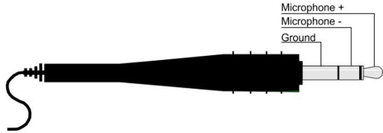
Figure 6: Microphone Pinout
