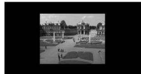
**FOLLOW OUTPUT** – The aspect ratio and resolution of the input signal is re-sized to precisely match the aspect ratio and resolution of the **VP-770** output signal. This may result in some distortion to the input signal images
