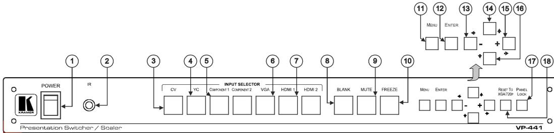
Figure 1: VP-441 Presentation Switcher/Scaler Front Panel
