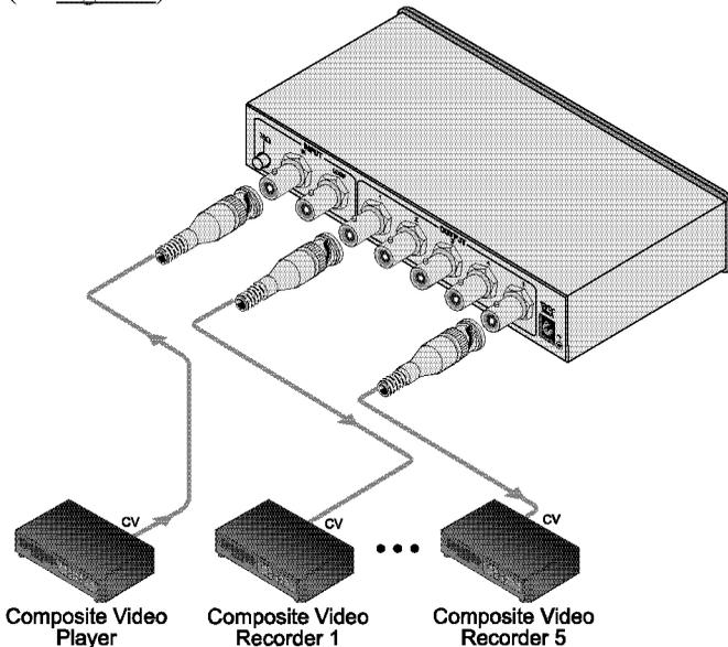
*Figure 9: Connecting the VM-50V 1:5 Video Distributor*
