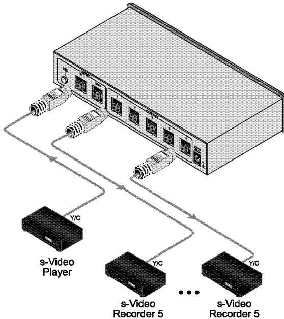
*Figure 10: Connecting the VM-50YC 1:5 s-Video Distributor*
