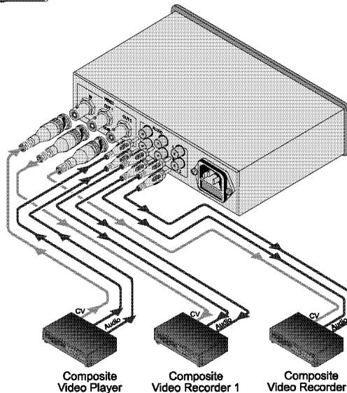
*Figure 6: Connecting the VM-2N Video Audio Distributor*
