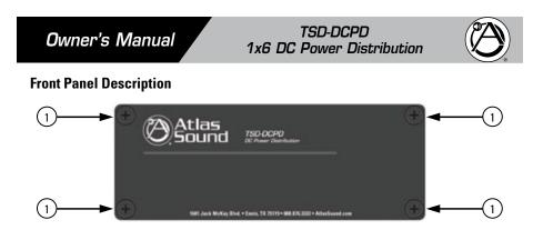
1. **Bracket Retainer Points** - Each TSD includes two mounting brackets for securing the TSD to a cabinet or wall. Remove screws and align the bracket with the panel hole before firmly tightening the screws.
