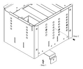
Figure 6: Installing the T-TBLANK TOOL Blank
