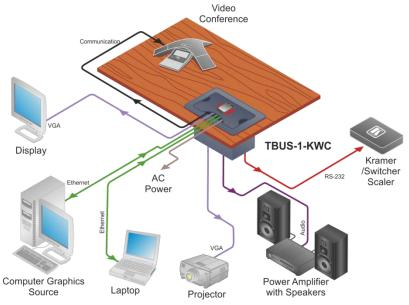
Figure 12: TBUS-1-KWC Boardroom Installation
