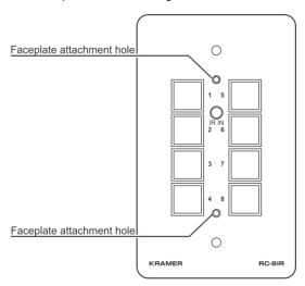
Figure 8: RC-8IR Faceplate Holes Table Connection Bus
