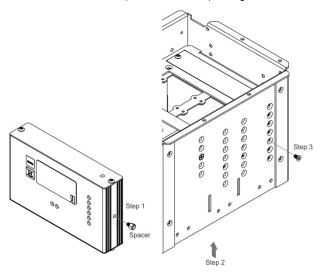
Figure 5: Installing a Kramer TOOL
