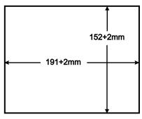
Figure 9: Cut Out Dimensions
