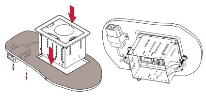
Figure 10: Inserting TBUS-1-KWC into the Prepared Opening
