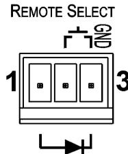
Figure 5: Remote Select Switch and LED Wiring
