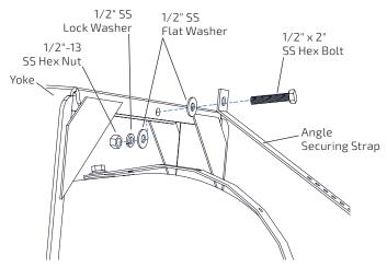
Figure 5a. Attach the securing strap to the yoke
