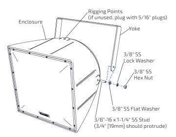
Figure 2. Mount the R.5-MAX loudspeaker to the yoke
