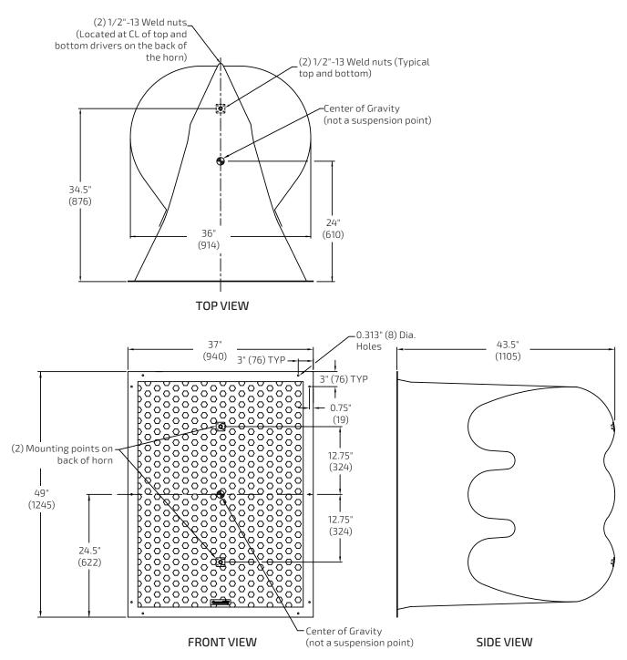
**Note:** Cabinets are handmade and measurements may vary slightly due to the thickness of the fiberglass. Dimensions shown should not be used to fabricate hanging fixtures. Mounting points are approximate.
