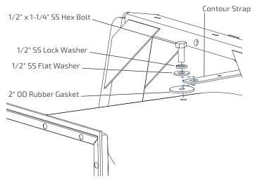
Figure 5b. Attach the contour strap to the enclosure
