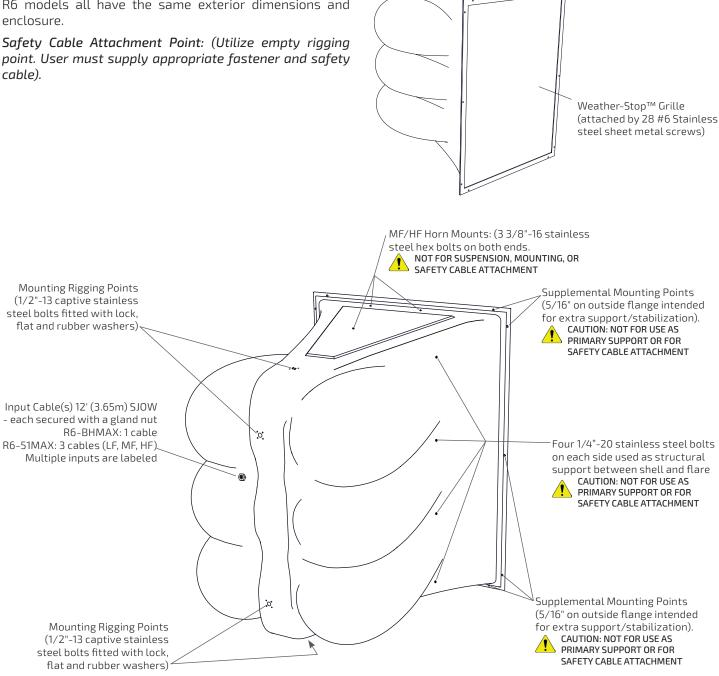
Note: Cabinets are handmade and measurements may vary slightly due to the thickness of the fiberglass.
