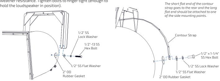
Figure 4a. Mount the R2-MAX loudspeaker to the yoke
