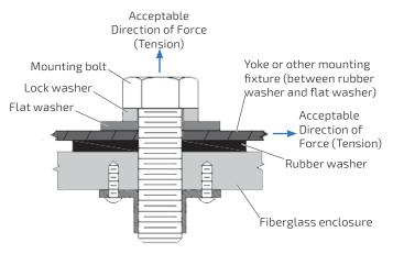
Figure 6. Mounting Point Loading
