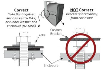
Figure 1. Mounting point load
