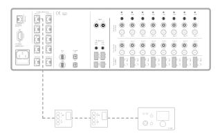
Multiple DW3018/4018 and one DW5065 Wall panel on one PI Port (PI1 to PI8)
