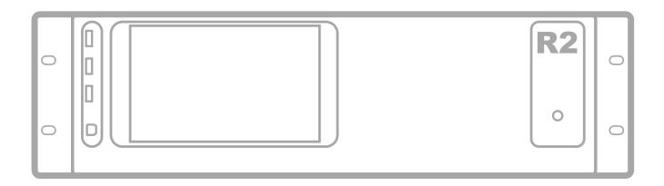
On the front of the R2 amplifier are a power button, four USB connection ports space for an optional touchscreen (R2DIS) provided.
