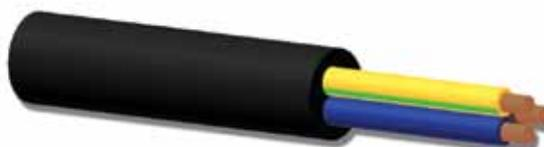
The PC3G15 and PC3G25 are high quality standard H05VV-F power cables for indoor and outdoor, fixed or mobile use. The cables are made of 3 PVC insulated conductors, with a diameter of 3 mm each (PC3G15) or 3,5 mm each (PC3G25) . These cables can be used in damp spaces.
