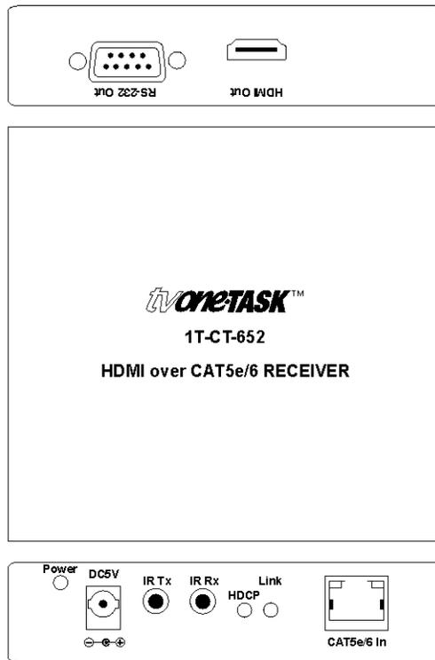
1. At the remote location, connect the Cat.5e/Cat.6 cable to the Receiver's RJ45 connector. Ensure that the connector achieves a positive lock into the receiver's connector.
