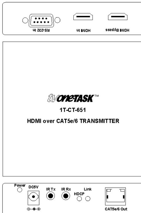
1. Connect the HDMI source device's output to the HDMI IN connector of the 1T-CT-651 Transmitter, using an appropriate HDMI cable, (1 Meter (~3') in length for 12 bit signals, 15 meters (~45') for 8 bit signals).
