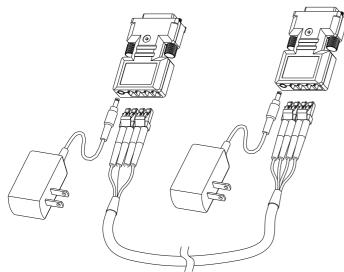
Figure 1 – Optical DVI Extension Modules System
