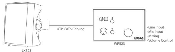
The LX523 is a 3-way stereo loudspeaker system consisting of an active and passive loudspeaker, designed to be used in combination with separate available (or as a set) input units such as the WP523 Wall panel and the RM523 Web based Input Control Unit. It is able to produce a clear and powerful sound with a power up to 2 x 40 Watt, offering a flexible solution for a wide variation of applications.
