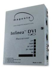
Magenta Research's Infinea<sup>TM</sup> is the ultimate solution for transporting DVI (Digital Visual Interface) signals over copper and/or fiber. Infinea can extend the reach of DVI sources over three different cable types. First, one strand of single mode fiber provides DVI long haul distances of 10 km (6.2 miles) or more. Second, dual multimode fibers carry DVI signals 500m/1640 feet. Third, a single Cat6 cable provides DVI transportation for short to medium distances (183 meters/600 ft.).
