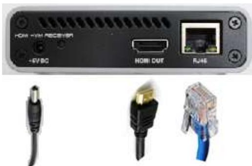
Power Jack (5V, 3.5mm)    HDMI Output (Monitor)    RJ45 JACK (LAN)
