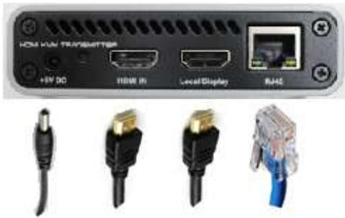
Power Jack (5V, 3.5mm)    HDMI Input (Source)    HDMI Output (Monitor)    RJ45 JACK (LAN)
