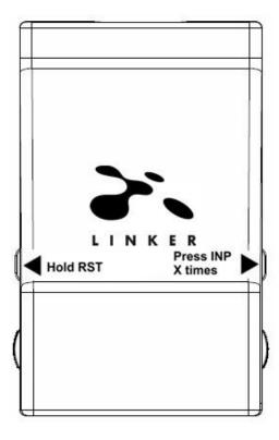
For users without access to GUI for Windows PC, we added a dual-button combo, when RESET is pressed down and INPUT is clicked the **CS** (Color Space) and **DC** (Deep Color) mode presets cycle between
