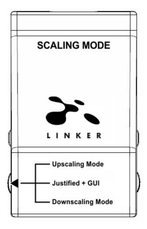
Scaling Mode slide switch has 3 positions.
