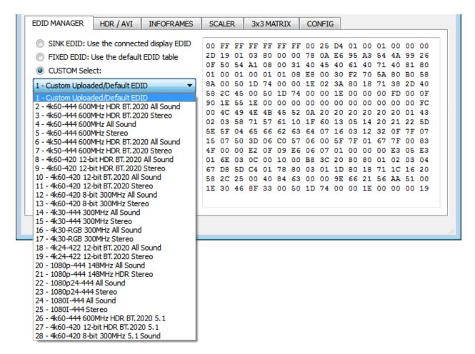
[SINK EDID Mode]: Create EDID based on the capabilities of the connected sink.
