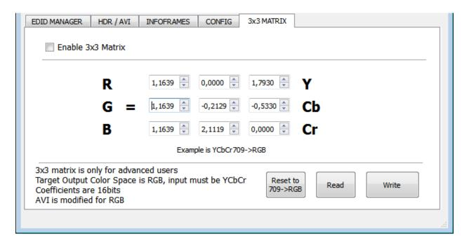
[Enable 3x3 Matrix]: Enable/Disable the 3x3 Matrix conversion.
