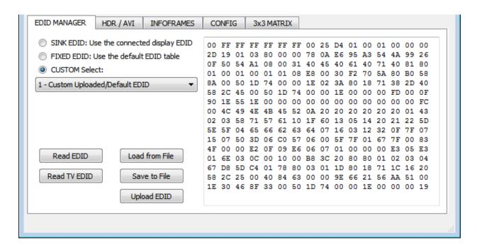
**Read EDID:** This option could be useful if for example you want to double check the build capabilities of an SINK EDID in your setup using external software such as <u>AWEE</u> (AW EDID Editor from Analog Way). In such case, you would simply use the **Read Linker EDID** button and then the **Save to File** button in order to be able to open the EDID file with an external EDID editor software.
