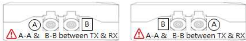
Fig Figure 3 – Fiber numbering & Caution on both fiber ports
