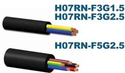
The H07RN-F3G1.5, H07RN-F3G2.5 and H07RN-F5G2.5 are high quality standard H07RN-F power cables for indoor and outdoor, fixed or mobile use. The cables are made of 3 (H07RN-F3...) or 5 (H07RN-F5...) soft rubber insulated conductors, with a diameter of 3 mm (...G1.5) or 3.5 mm (...G2.5). Packed in a highly flexible rubber outer jacket of respectivly 9 mm , 11 mm and 14 mm.
