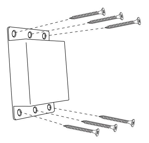
The Gefen *DVI Galvanic Isolator* can be mounted on any flat surface using wood / drywall screws as shown in the diagram above. There should be an inch or two of clearance between the edges of the unit and any walls or vertical surfaces to allow for enough clearance for connection and disconnection of DVI cables.
