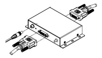
**IMPORTANT**: The Grounding Stud must be permanently connected to protective ground by wiring not less than 16 AWG.
