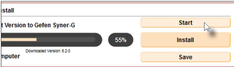
After the **Start** button is clicked, the Syner-G software will automatically download the latest firmware and begin updating the matrix. The update process will be indicated by the progress bar.
