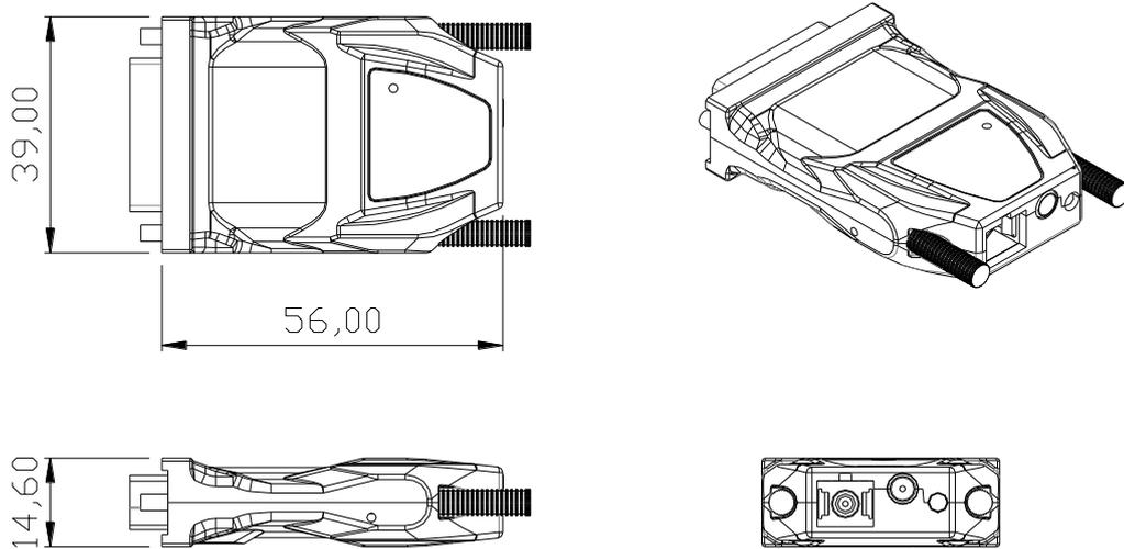
Note: The transmitter, DVFX-100-T and the receiver, DVFX-100-R have the same mechanical dimensions.
