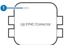
**1 POWER LED:** The LED will illuminate in blue when the power is connected.
