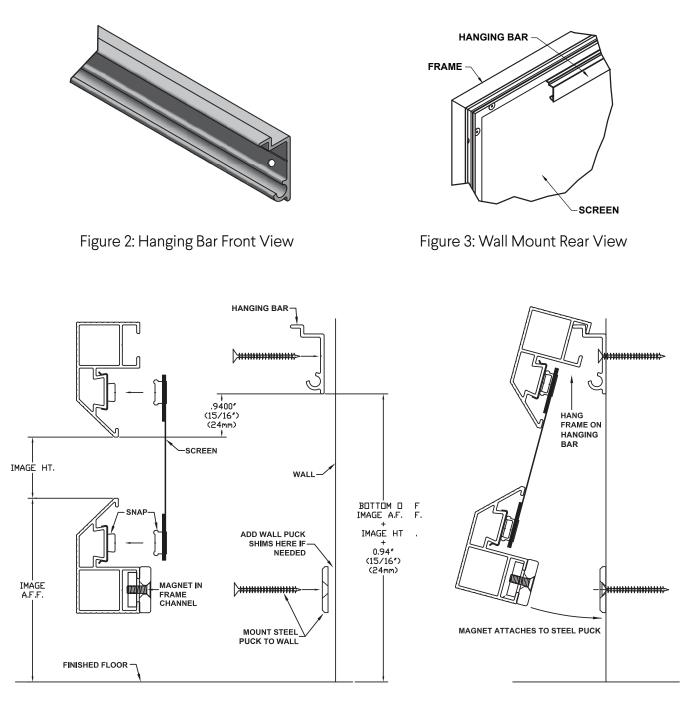
Figure 4: Components for Wall Mounting - Side View
