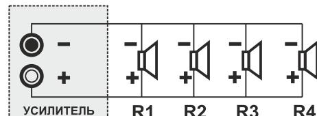
$$1/R = 1/R_1 + 1/R_2 + 1/R_3 + 1/R_4$$
