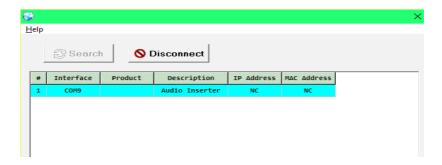
After launching the software, power the unit on and then connect it to the PC/laptop using a USB cable. Click on the "Search" button and any detected units will be displayed in the list. Clicking on a detected unit will open the EDID Commander window.
