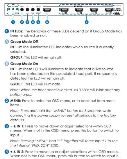
Note: Pressing "MENU" and "+" together will force Input 2 to use the Internal "FHD, 2CH" EDID.
