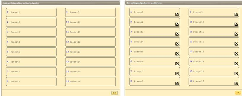
This unit can store up to 16 routing presets. Presets can be utilized to store multiple different routing states in advance for rapid, hassle-free, recall.
