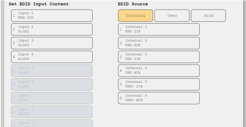
3) **Set EDID Input Content/EDID Source:** The Set EDID Input Content section allows for the assignment of a specific EDID to any supported input port. Click on one or more input buttons on the left, select the EDID category (Internal, User, or Sink), then select the new EDID source to use from the choices on the right. The buttons will change color as you select them and the EDID change will occur immediately across all selected Inputs.
