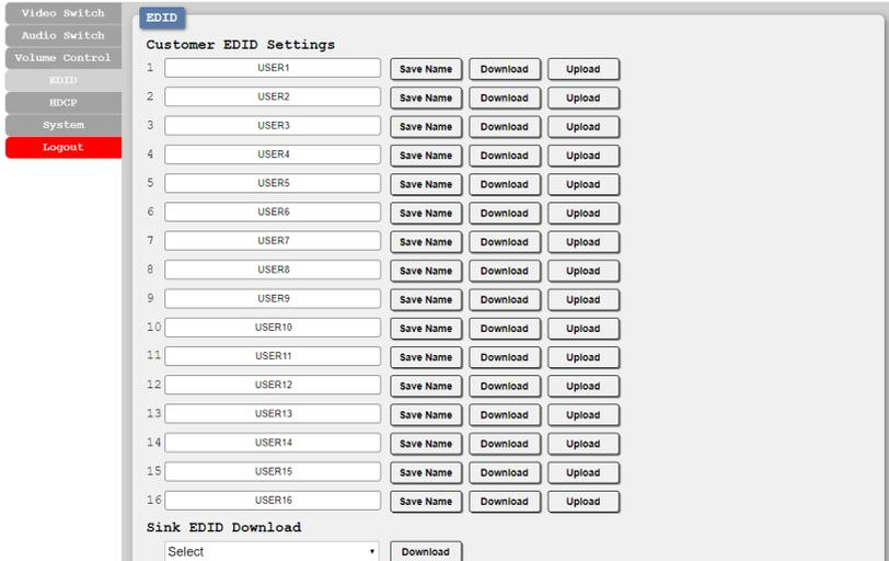
The screenshot shows the EDID configuration interface. On the left is a sidebar with navigation options: Video Switch, Audio Switch, Volume Control, EDID (selected), HDCP, System, and Logout. The main area is titled 'EDID' and contains 'Customer EDID Settings' with 16 rows, each with a text input field (USER1-USER16), a 'Save Name' button, a 'Download' button, and an 'Upload' button. Below this is a 'Sink EDID Download' section with a dropdown menu labeled 'Select' and a 'Download' button.
