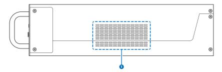
1 VENT FAN: These vents are for are for air ventilation. Please allow adequate space around the unit for air circulation.
