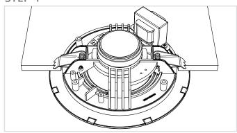
Insert the speaker through the provided ceiling cutout, make sure the spring loaded mounting arms are behind the clamping surface and release them. The ceiling is clamped between the mounting arms and the speaker baffle and is installed correctly.
