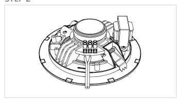
Connect the wires coming from the amplifier to the terminal block connector on the rear of the loudspeaker.
