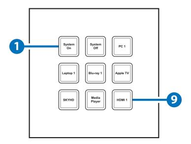
1 1~9 Macro Buttons: Each buttons has 2 colors of LEDs adjustable from dim 0~100% and can be insert up to 16 commands.
