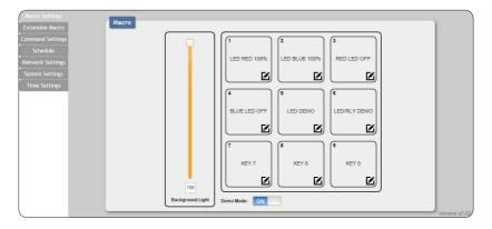
The Background Light Bar allows user with instant change on the LEDs lighting percertanage base on the original illuminate setting.
