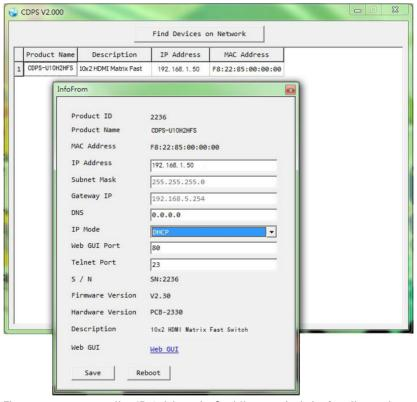
Then user may use the IP Address to find the control device through Telnet, WebGUI or even RS-232/Hyper Terminal tools.
