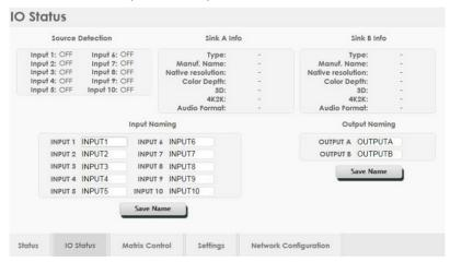
Click on IO Status to view connection status and output EDID information and to rename input and output ports.
