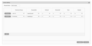
Once the Preset settings window is open, the name of the Preset can be set at the top of the window. Pressing the "Add" button will add an additional Receiver/Group routing line. To delete an existing route, click on the "Remove" button next to the route to remove. Once all routes for the Preset have been defined, press the "Confirm" button to save the changes. Each route line has the following configurable settings:
