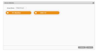
The name of the Display Group is set at the top of the window. To add Receivers to the Display Group, click on the name of each one to include. To remove a Receiver from the group, click on the Receiver's name a second time. After all selections have been made, click on the "Confirm" button to save the changes.
